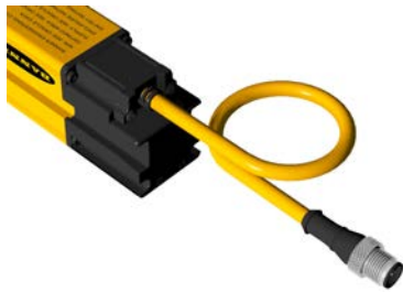
Figure 5. 300 mm Pigtail with M12/Euro-style QD
